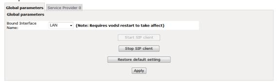
**Bound Interface Name**: Select the interface to use for the voice service, for example: ppp\_0\_8\_35\_2.
