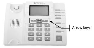
To enter selected menu function press left arrow key  $\blacktriangleleft$  (LCD displays OK), to exit press right arrow key  $\blacktriangleright$  (LCD displays Exit).
