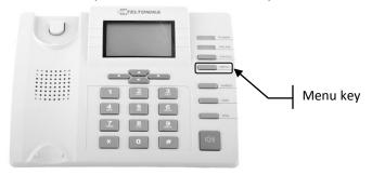
Menu items are selected by using up and down arrow keys  $\blacktriangle \ lacktriangledown$  located below the LCD screen.
