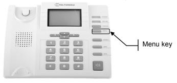
Menu items are selected by using up and down arrow keys ▲ ▼ located below the LCD screen.
