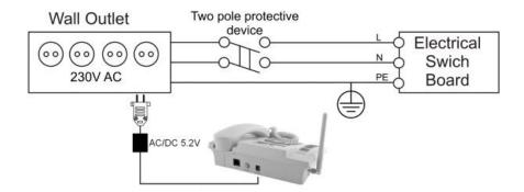
Signal level of the device depends on the environment in which it is working. If the device starts working insufficiently only qualified personnel may repair this product. We recommend to send it to repair centre or to manufacturers. There are no exchangeable parts inside of the device.
